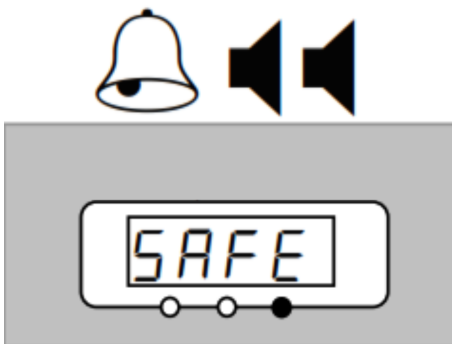
Fig. 7: Excess temperature alarm
